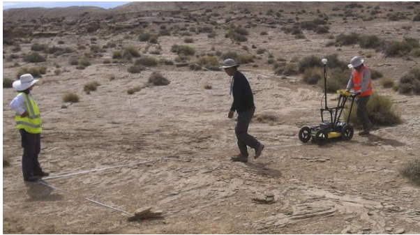
Figure 5: Rectangular grid (25 m x 15 m) of 3D GPR data acquisition using Sensors and Software's Noggin Plus SmartCart 250 MHz antenna on the top of the outcrop analog.
